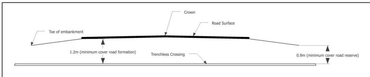
**Figure 5.2.2(b) – Minimum depth below dual carriageway**
