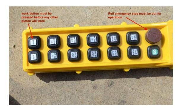
The red emergency stop button must be out for the pendant to work.
