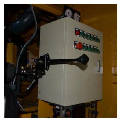
(Pressure / Vacuum (4way) valve lever (option) UP (45°) - Pressure Middle (Horizontal) - Neutral Down (45°) - Vacuum Press Button - UNLOCKS LEVER Release Button - LOCKS LEVER
