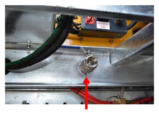
Water Tank Drain Valve Lever
